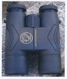
The KOC 10x42F is a typical, modern roof prism binocular with twist-up eyecups and a conveniently located centre focus wheel. The rubber armour coating is textured to provide a nonslip grip. Given the boomerang motif on each barrel, you could almost be tempted to think the binocular was made for Australia.
